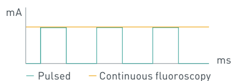
Intelligent pulse technology based on short, sharp pulses minimizes dose exposure and maximizes image quality.
