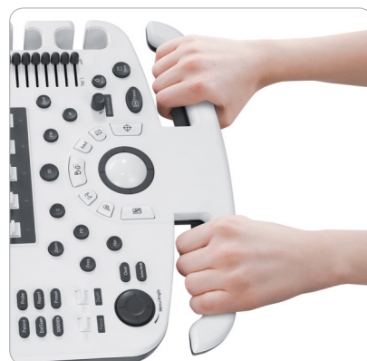
Lifting Control Panel
